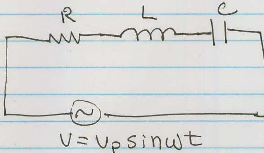
Objective 1. To determine the phase angle " $\phi$ " between the current and applied voltage.
